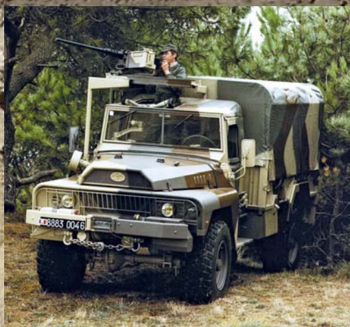
ABOVE: the VLRA TPK 4.25 SH is a shelter carrying variant with a payload of 2400 kg.
