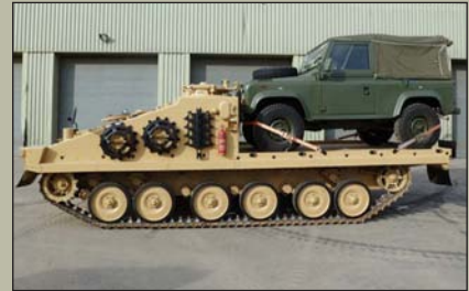
Alvis CVRT Shielder , Tracked Armoured load carrier with flat bed platform, The flat bed can adopted for a wide range of roles such as logistic carrier, bridge layer repair / recovery and towing. Built to a high specification the vehicle hull is composed of aluminium armour to protect the crew, etc, Mileage from 500, Excellent condition, Guide price from £15,000 (20 Available) .
