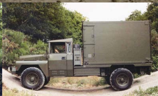
ABOVE: the VLRA TPK 4.25 SH is a shelter carrying variant with a payload of 2400 kg.
